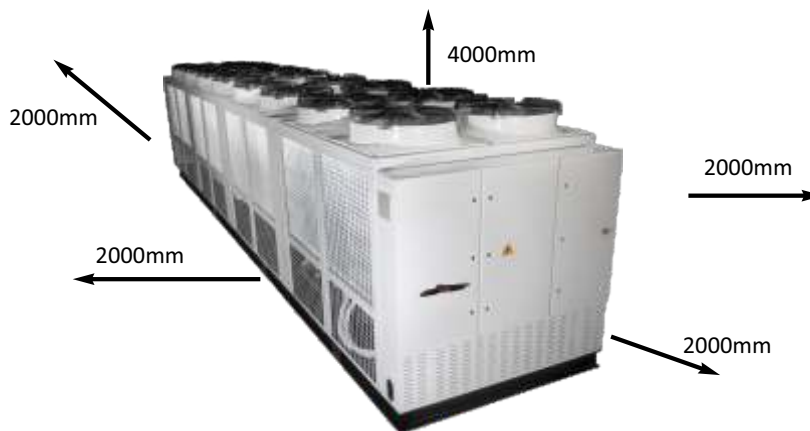
b. Installation and service space required for more than one chiller.
